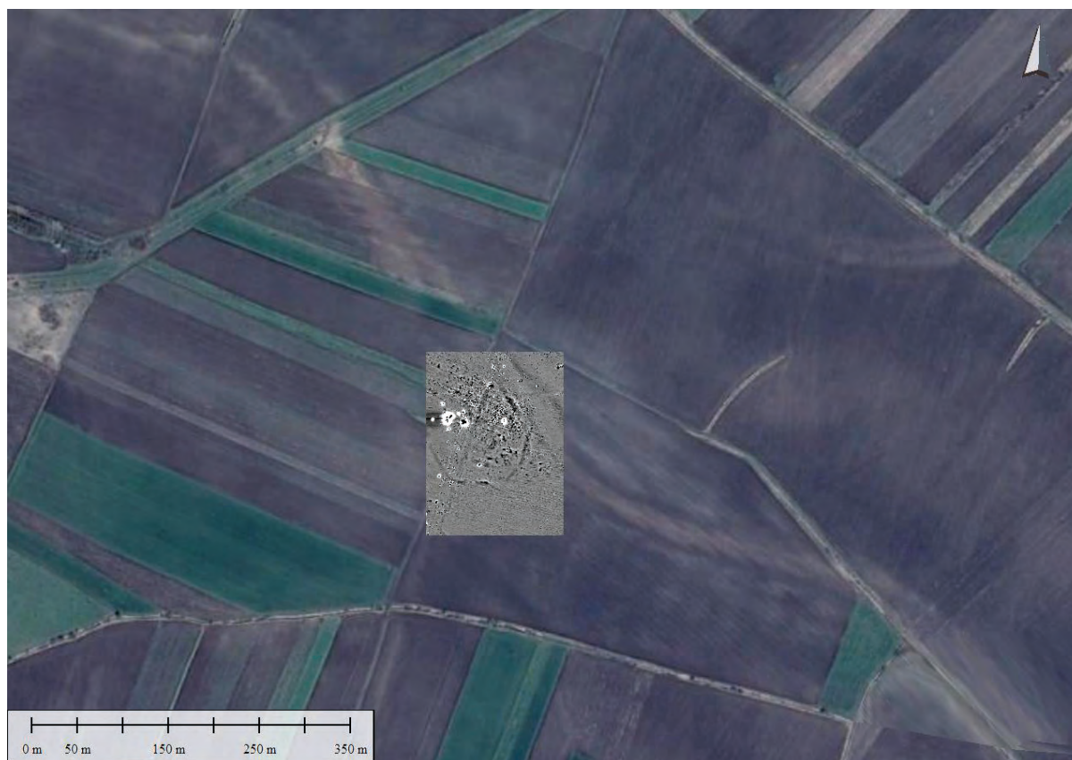
Fig. 16. Berveni-Holmoș. Greyscale plot of the magnetometer survey overlying the satellite image (source: Google Earth).
